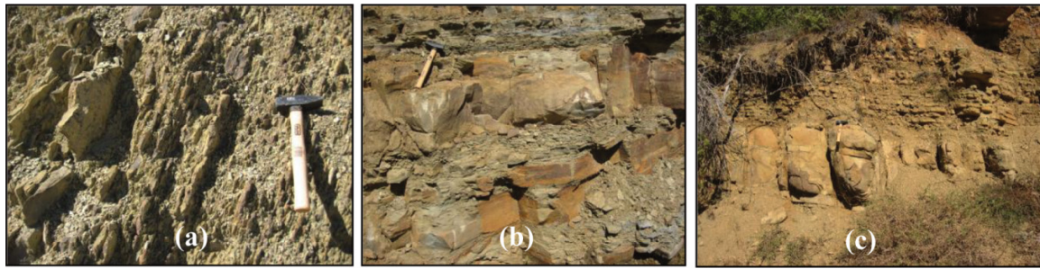
Fig. 3. (a) Examples of thin-bedded alternations of siltstones and sandstones from Mt. Driskos region (folding of the formations is evident in part (c)). (b) Medium- to thick-bedded sandstones and thin-bedded siltstones; shear zones exist along the bedding planes and the fracturing (faults) along axial plains. (c) Thick-bedded sandstones with alternations of thin-bedded siltstones.
