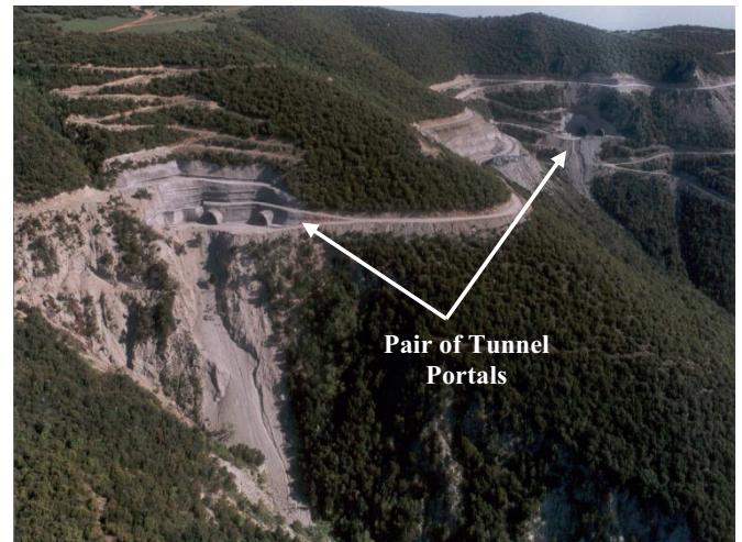
Fig. 2. Portals of tunnels of Egnatia Odos Highway depicting the nature of the challenging geological conditions.
